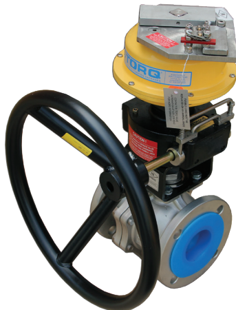
FLP-HT series fusible link shown with 4" stainless steel flanged ball valve NOTE: The FLP-HT Series incorporates a declutchable manual override to arm and operate the assembly.
